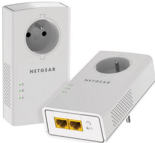
NETGEAR Powerline 2000 + Extra Outlet - - adaptateur CPL - - 1GbE, HomePlug AV (HPAV) 2.0 - Branchement mural (pack de 2) test
